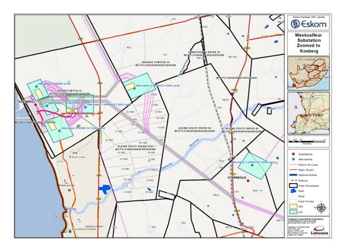
**Figure 3.7:** The 5 alternative sites within the study area (Note that the extent of the Air Insulated Substation (AIS) on the map is larger than required at 950 x 750 m, the actual required size is  $760 \times 550$  m)
